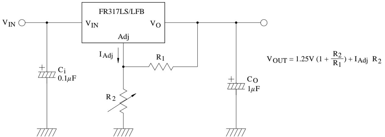
$C_i$  is required when regulator is located an appreciable distance from power supply filter.
