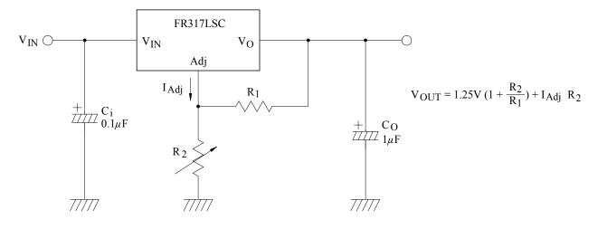
Ci is required when regulator is located an appreciable distance from power supply filter. Co is not needed for stability, however, in the range of  $1\mu$ F to  $100\mu$ F of aluminum or tantalum electrolytic are commonly used to provide improved output impedance and rejection of transients. Since  $I_{Adj}$  is controlled to less then  $100\mu$ A, the error associated with this term is negligible in most applications.
