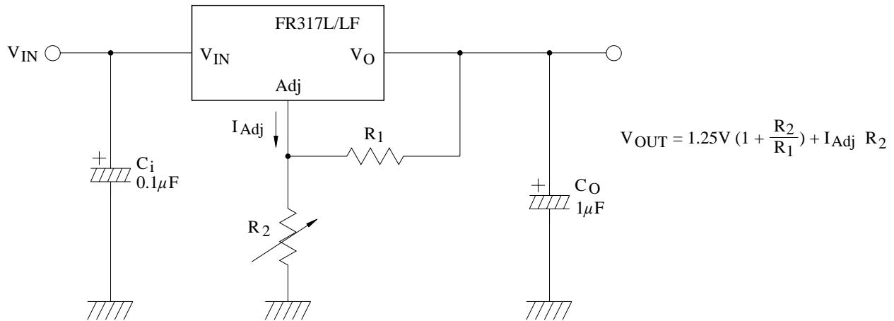
$C_i$  is required when regulator is located an appreciable distance from power supply filter.
