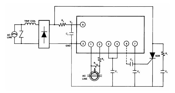
Supply voltage circuit is connected as a previous diagram. Please decide constants R1, R2, C4, and C5 of a filter in order to keep at least 12V in V+, when normal supply current flows.
