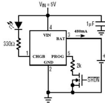
Li-ion Charger with External Power Dissipation
