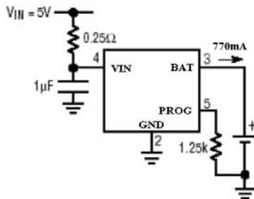
Basic Li-ion Charger with Reverse Polarity Input Protection
