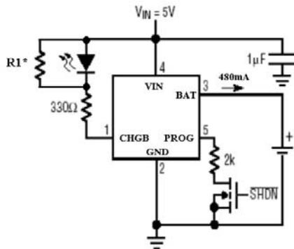
\*The formula for R1 is  $R1 < \frac{V1}{35\mu A}$ , where V1 is the turn-on threshold voltage of the LED device.
