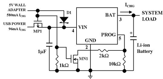
**Figure 5. Combining Wall Adapter and USB Power**
