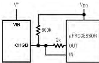
**Figure 3. Using a Microprocessor to Determine CHGB State**
