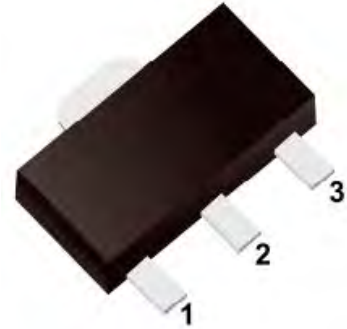
1. Base 2. Collector 3. Emitter SOT-89 Plastic Package
