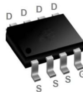
SOP-8 Pin Configuration
