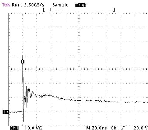
Figure 1. ESD Clamping Voltage Screenshot
