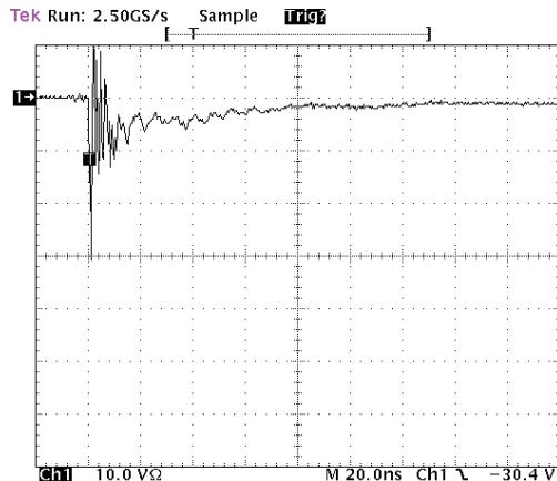
Figure 2. ESD Clamping Voltage Screenshot
