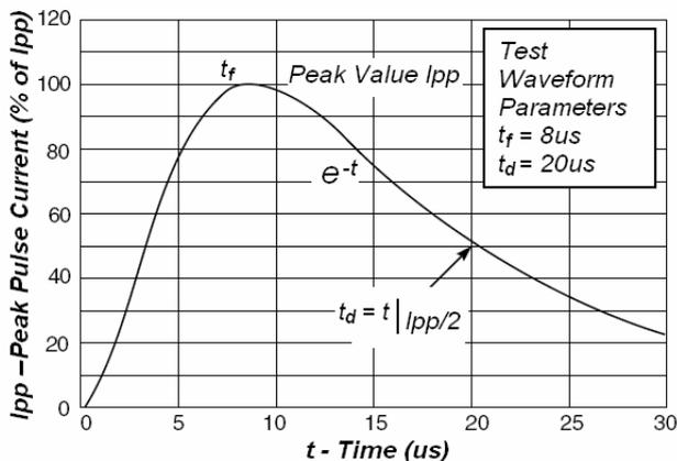
Fig1. Pulse Waveform
