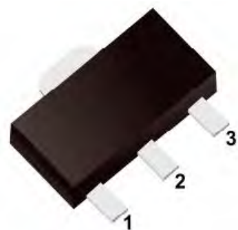
1. Base 2. Collector 3. Emitter SOT-89 Plastic Package
