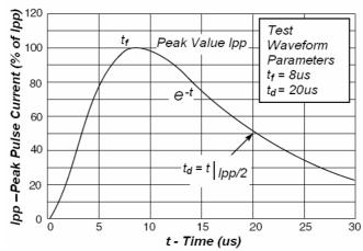
Fig1. Pulse Waveform
